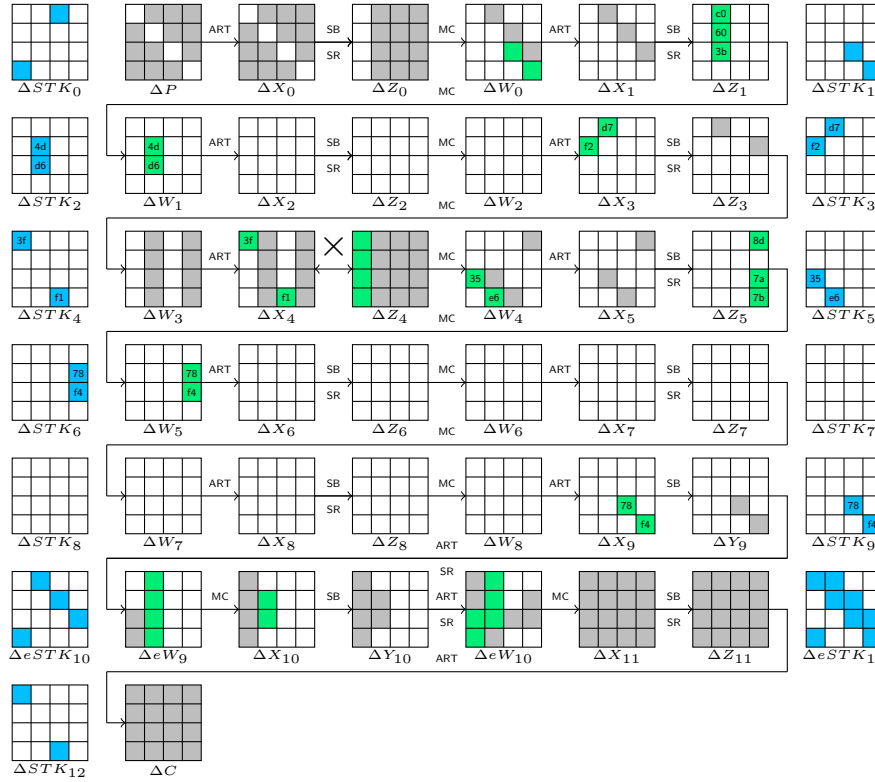
Figure 13: 12-round related-tweakey impossible differential attack against Deoxys-BC-384
