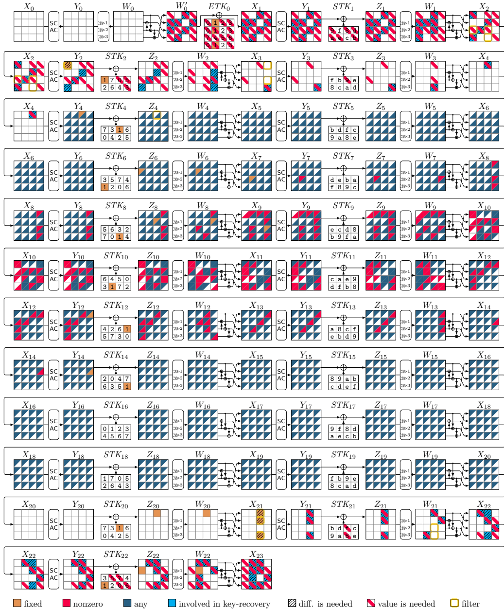
Figure 42: Related-Tweakey ID attack on 23 rounds of SKINNY128-288-128. |k_B \cup k_F| = 120 , c'_B = 56 ( c_B = 48 ), c_F = 40 , \Delta_B = 56 , \Delta_F = 40 . In this case, we have 255 related-key impossible differences.
