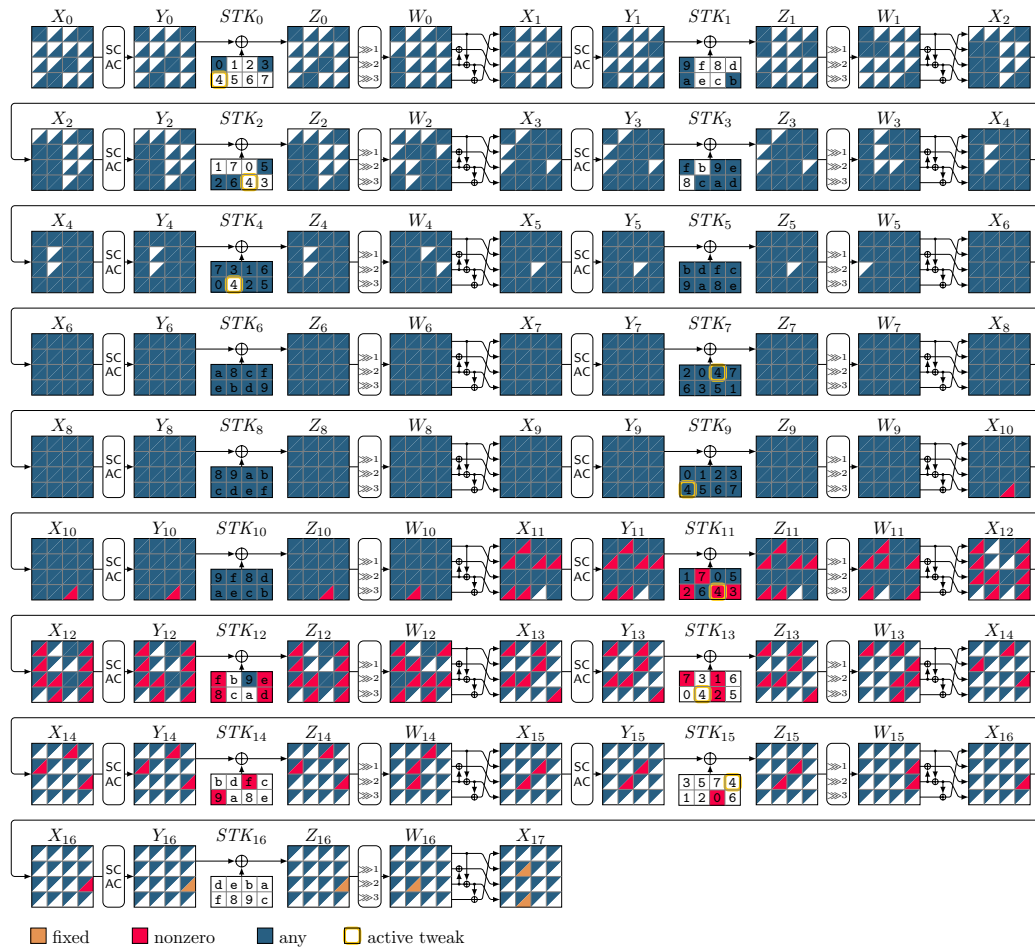
Figure 26: Integral and ZC distinguishers for 17 rounds of ForkSKINNY-64-192, where r_i = 6 , r_0 = 23 , and r_1 = 11 .
