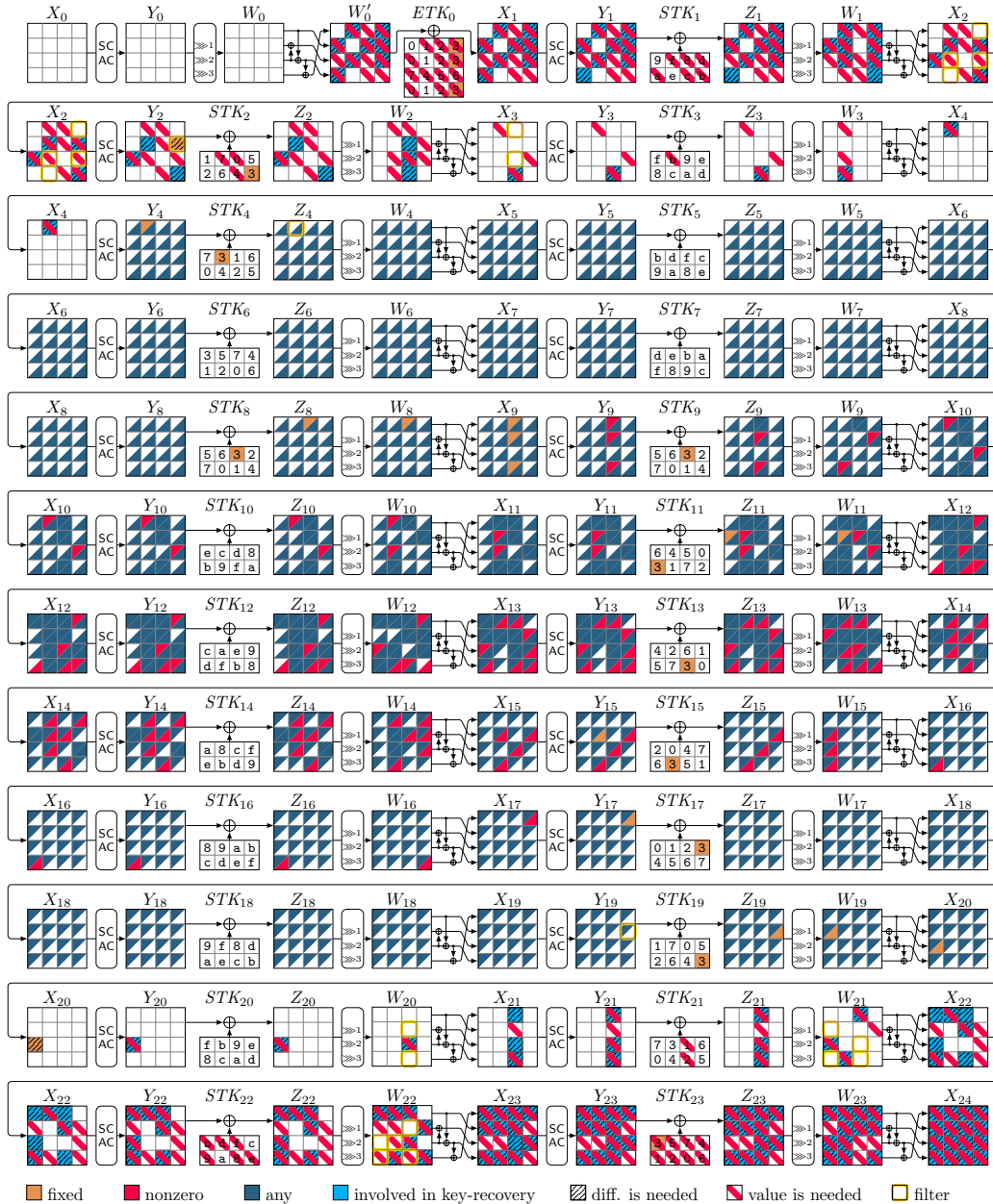
Figure 35: Related-Tweakey ID attack on 24 rounds of ForkSKINNY-128-256-256 in the limited setting ( r_i = 9, r_0 = 15 ). |k_B \cup k_F| = 224 , c'_B = 64 ( c_B = 56 ), c_F = 96 , \Delta_B = 64 , \Delta_F = 96 . In this case we have 15 related-key impossible differences.
