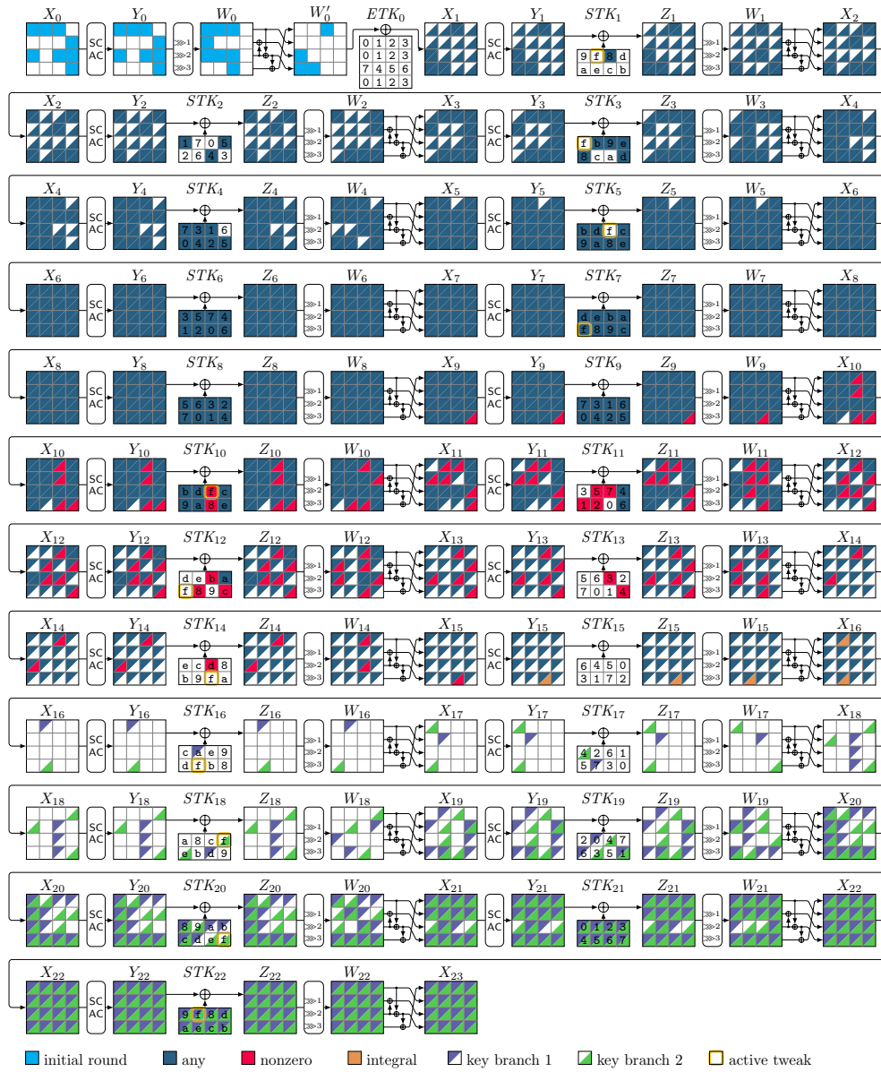
Figure 19: ZC-based integral attack on 23 rounds of ForkSKINNY-128-256.
