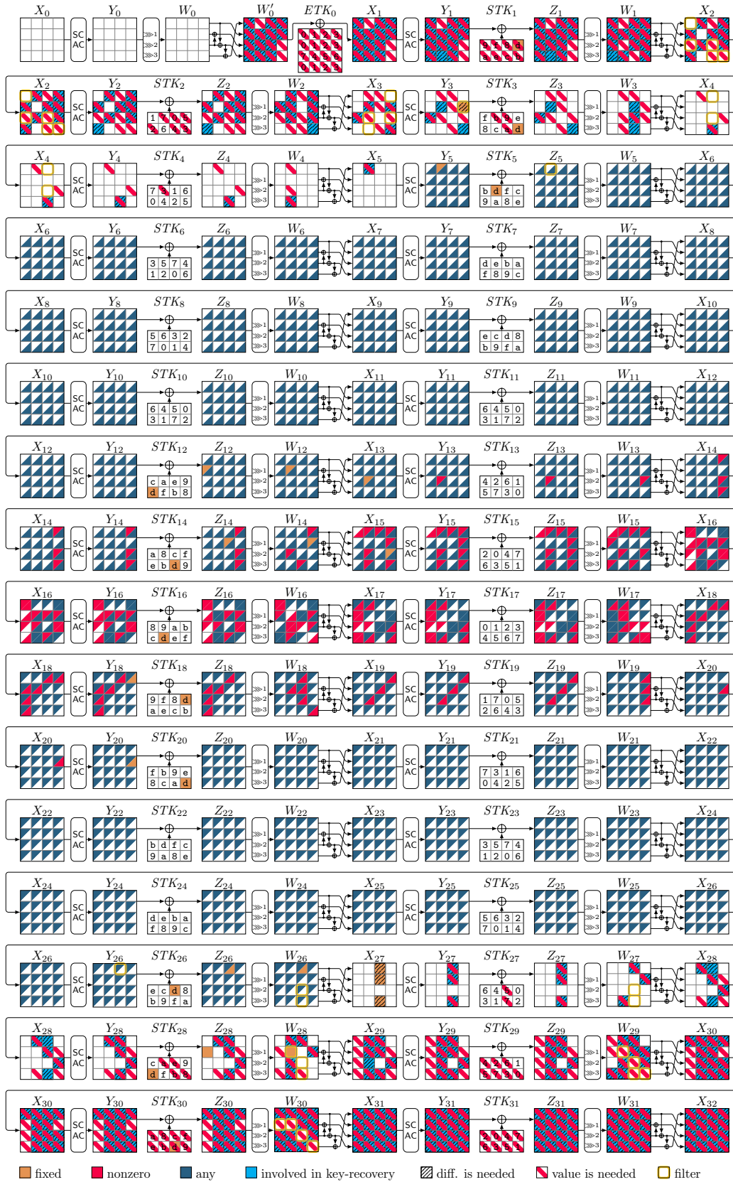
Figure 31: Related-Tweakey ID attack on 32 rounds of ForkSKINNY-64-192-192 in the arbitrary setting ( \mathbf{r}_1 = 11, \mathbf{r}_0 = 15 ). |k_B \cup k_F| = 176 , c'_B = 52 ( c_B = 48 ), c_F = 64 , \Delta_B = 52 , \Delta_F = 64 . In this case we have 15 related-key impossible differences.
