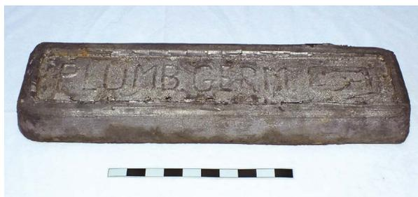
Figure 18. Modern lead ingot with cartouche inscription from a wooden model. Photo: I. Pfeffer.
