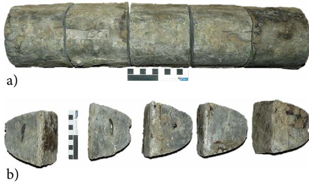
Figure 23. Roman lead ingot (a) from the northwest coast of Sardinia; (b) modernly divided with closed blowhole. Photos: N. Hanel.
