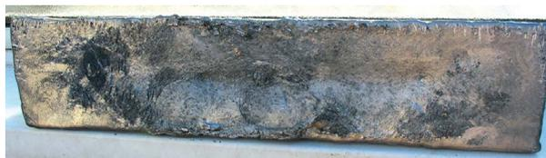
Figure 22. Modern ingot with a shrinkage cavity on the underside. Photo: N. Hanel.
