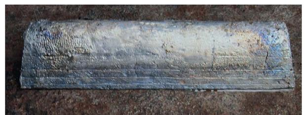
Figure 16. Modern lead ingot with an impression of the tissue remains (top left) and casting lines. Photo: R. Köhne.
