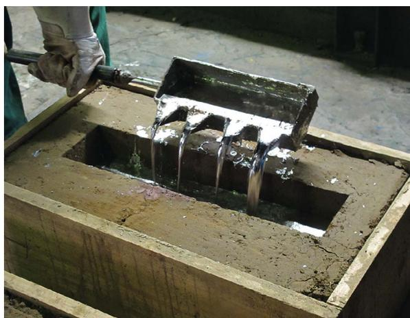
Figure 8. Pouring the liquid lead into the clay mould, using a metal four-pronged casting ladle. Photo: N. Hanel.
