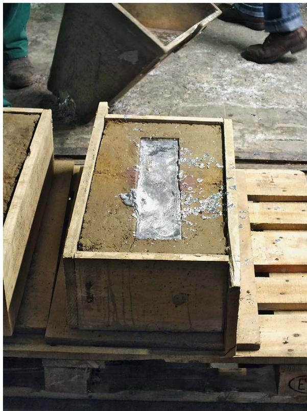
Figure 12. Finished lead casting into the clay mould - with bumps and small voids on the later underside of the ingot. Photo: I. Pfeffer.
