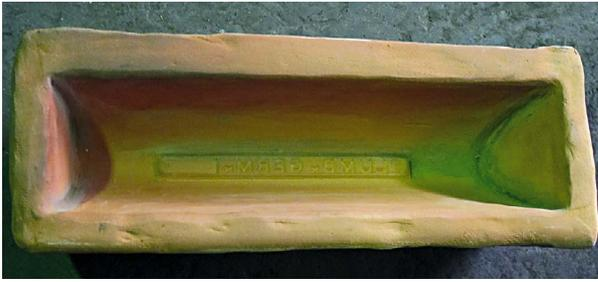
Figure 19. Modern ceramic casting mould of a lead ingot type A with inscription PLUMB GERM. Photo: R. Köhne.
