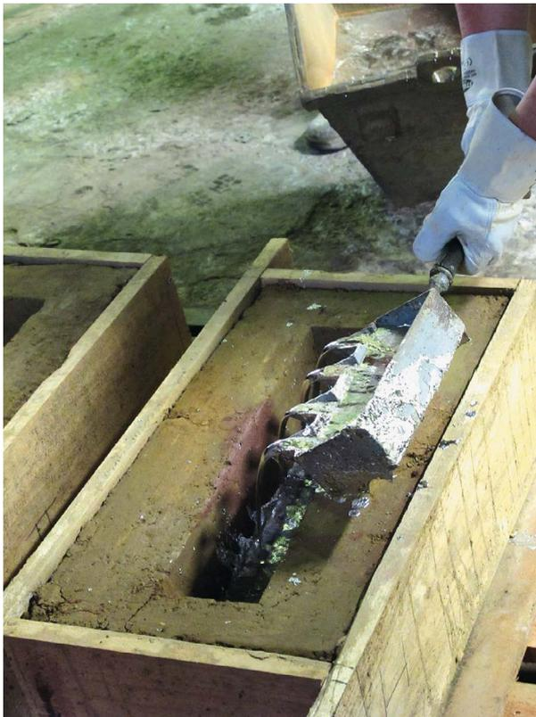
Figure 11. Pouring the molten lead into the clay mould, using a four-pronged casting ladle. In the background there is the metal vessel for removing the lead. Photo: N. Hanel.
