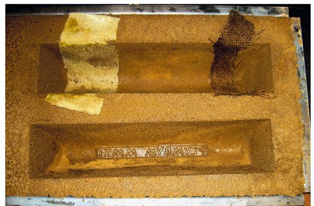
Figure 15. Clay mould for double ingot casting. Scraps of tissue inserted into the upper ingot. Photo: R. Köhne.
