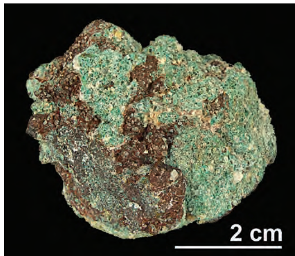
Figure 5: Nodule of a copper ore from Wadi Amram. The nodule is an impregnation of secondary copper minerals in sandstone. The brown colored core consists of a mixture of iron-bearing minerals, and cuprite may be present. It is covered by an incrustation of green copper minerals mainly consisting of malachite and atacamite.
