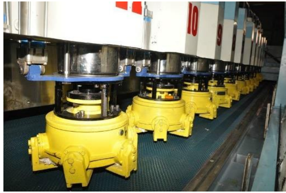
Fig. 1. Typical multiple head polishing machine used by the ornamental stone industry. [4]
